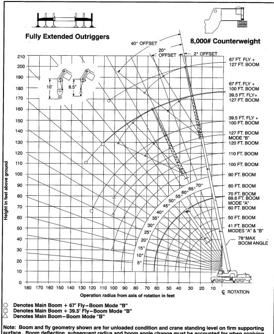
surface. Boom deflection, subsequent radius and boom angle change must be accounted for when applying load to hook.
