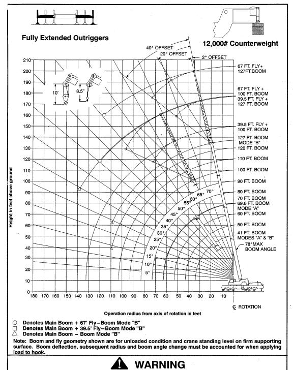
Do Not Lower The Boom Below The Minimum Boom Angle For No Load Stability As Shown In The Lift Charts For The Boom Lengths Given. Loss Of Stability Will Occur Causing A Tipping Condition.
