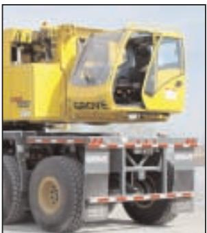
The new superstructure cab stows to the rear and swings hydraulically to the right side of the crane for operation. Stationary heating and A/C are standard.
