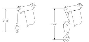
Dimensions are for largest Grove furnished hookblock and headache ball, with anti-two block activated.
